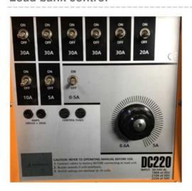
Steps of 5/10/20 / 30A + wheel for load from 0.5 to 5A
