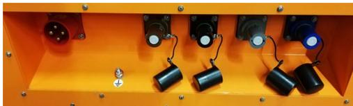
100 / 200 kW Connection: 1 cable by phase + ground
