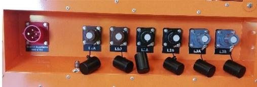
200 / 300 kW Connection: 2 cables by phase + ground
