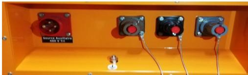
200 kW Connection : 1 cable by phase + ground
