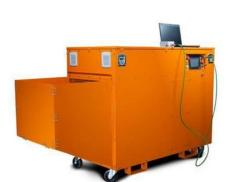
The SMART & connected function of our equipment allows you to control a whole fleet of load banks remotely via a single supervision PC. You will also be able to send them instructions and collect extremely precise data during your tests (P/U/I/ Delta T), which will allow you to:
